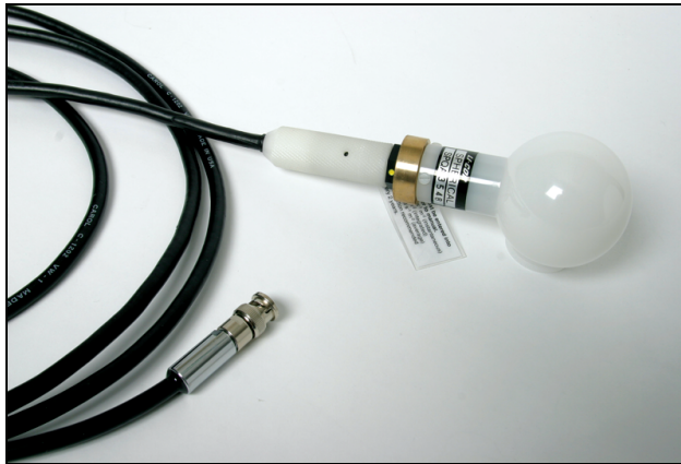
Figure 1-1. "SA" type sensors are terminated with only a BNC connector on the end of the coaxial cable.
