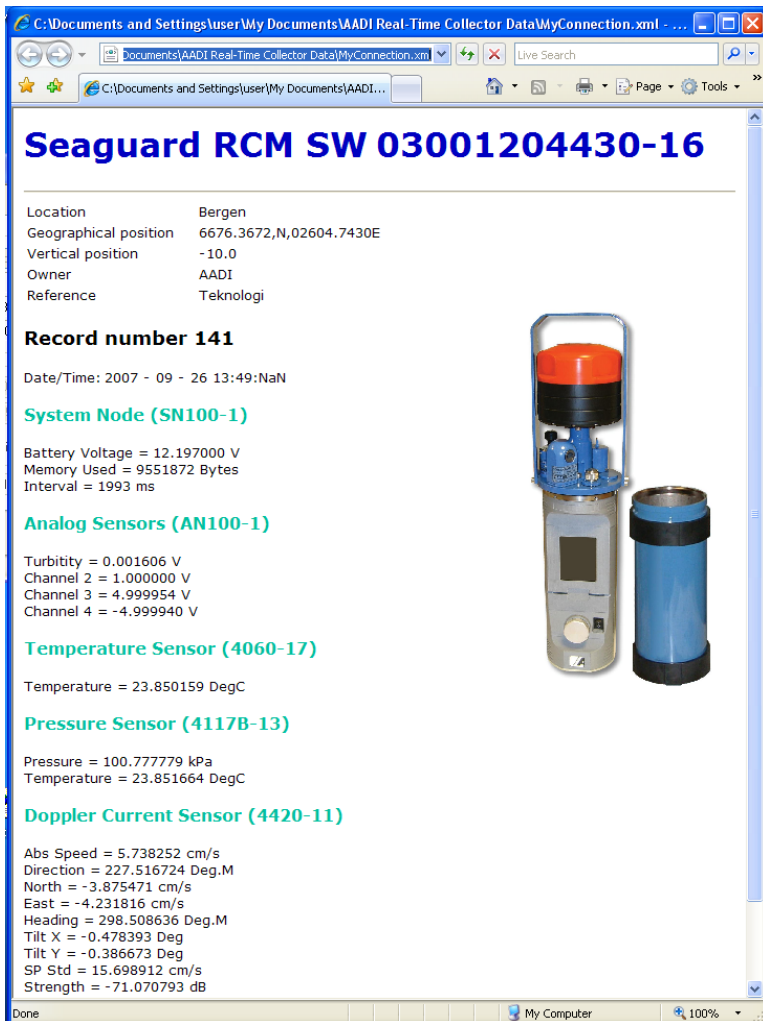
Figure 8-3 Viewing the xml file by using a style sheet to format the output.
