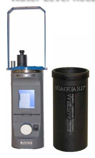
The SEAGUARD® Water Level Recorder measures hydrostatic pressure based on a silicon pressure sensor 4647. The pressure measurements are sampled and temperature compensated by an advanced Digital Signal Processor.
