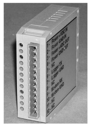
This Module provides an Isolated Electrical Serial Line between to types of Equipment regardless of the two Systems Ground or Main Supply Voltages and Electrical Potentials.
