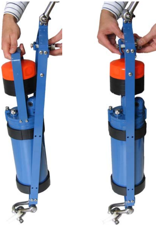
Figure 7-6 Mount the instrument into the frame.
