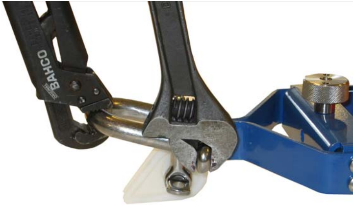
Figure 7-3 Fasten shackle in frame. Tighten thoroughly.
