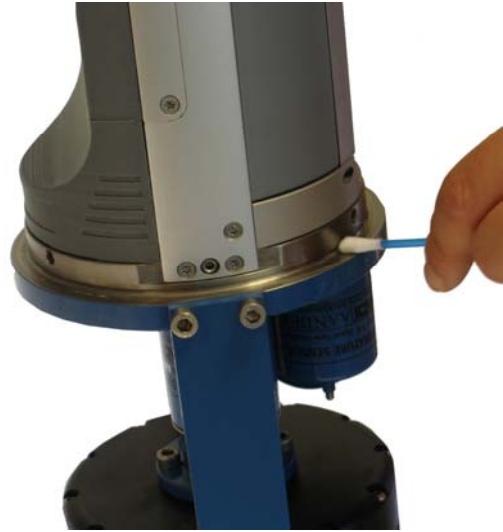
Figure 8-2 Clean O-ring seating; instrument up-side-down.
