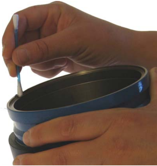
Figure 8-1 Clean O-ring seating.
