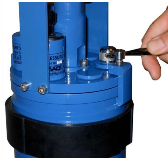
Figure 7-2 Tighten C-clamps until the pressure case rotates on the floor. Avoid over tightening as this will bend the C-clamps.
