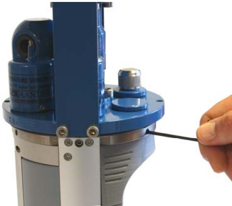
Figure 8-3 Fasten the set screws before putting on new O-ring.
