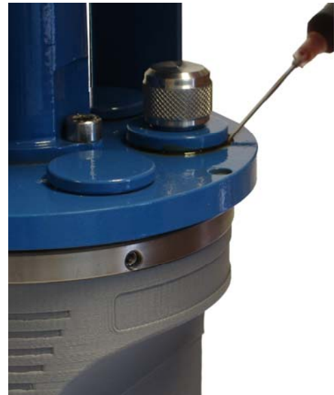
Figure 8-5 Add Tectyl® around sensors and sealing plugs.
