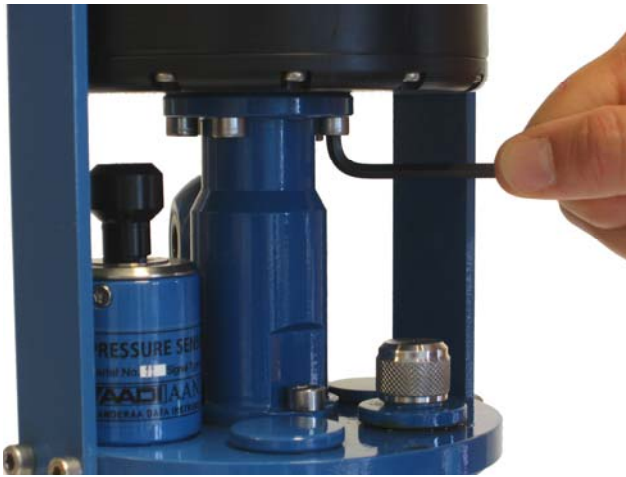
Figure 7-15 Connect the ZPulse™ DCS for the SEAGUARD® RCM.
