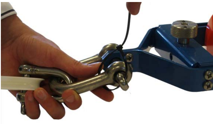
Figure 7-5 Lock the shackle with strips or locking wire. Locking wire is recommended for higher security in long deployments.
