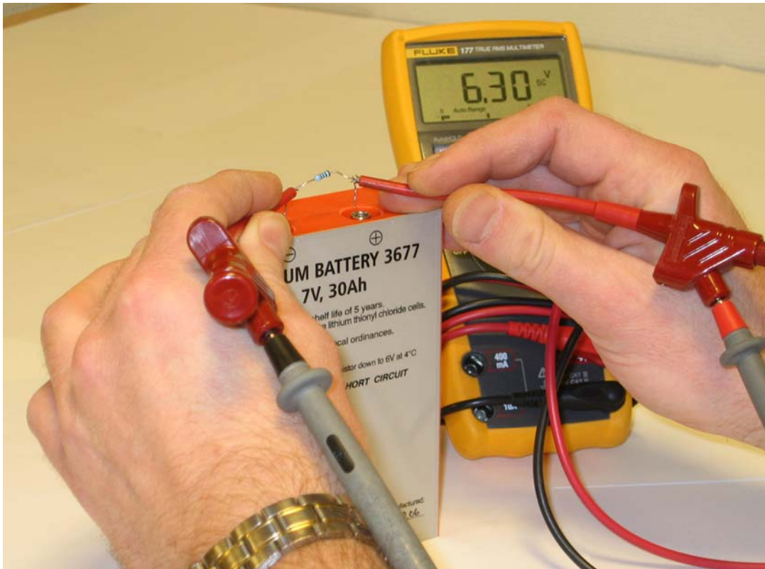
Figure 7-18 Use a 100 \Omega resistor up to 6.3 V to rejuvenate the battery.
